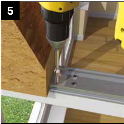
Fix the gable frame stiffener to the aluminium beam fixing plate using 4 x RRR025. Secure along the length of the stiffener at 500mm centres into frames (fixings not supplied). Set out image 7 page 46.
