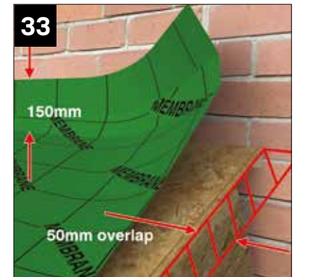
Cut the breathable membrane underlayer to the width of the roof deck plus 50mm over hanging the OSB barge-board at each end and 150mm up the host wall.
