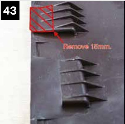
If obstructed on the RHS, remove 15mm from the clips to allow fitting.
