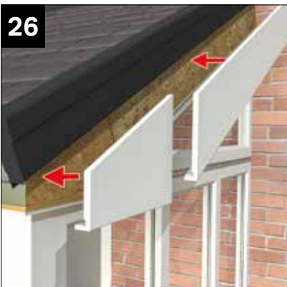
Fit the pre-cut fascia and eaves trims. See page 50, images 44 to 47 for more detail.
