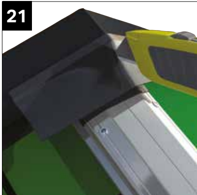
Fit second 200mm Butyl tape sealing the dry verge to the gable flashing. Cut the tape to allow it to be folded as shown in the following two images
