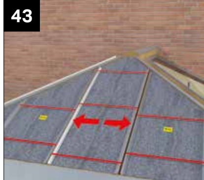
The expandable panel will expand to take up any tolerance gap. Snip the binding cord on all the remaining front facet panels.
