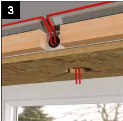
At lower pitches, when only one batten is fitted, the hole (and grommet) are positioned lower on the vertical face and the batten split to allow cable access.
