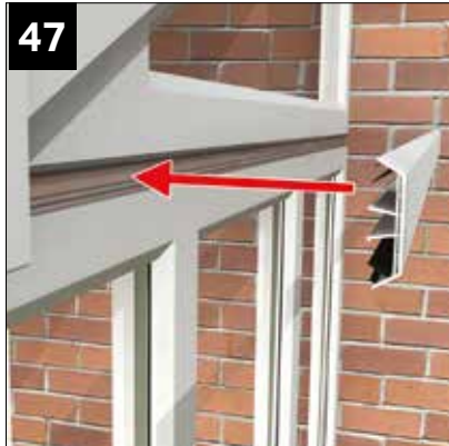
Fit internal and external gable stiffener claddings (if ordered). NOTE: Aluminium stiffer and cladding may need notching/ routing for frame drainage.
