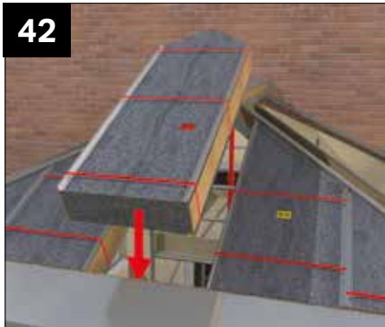
Lower into position the front facet central expandable panel. Marked with a red label.
