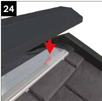
Fit the ridge top capping using the NRRSA 005BL supplied.
