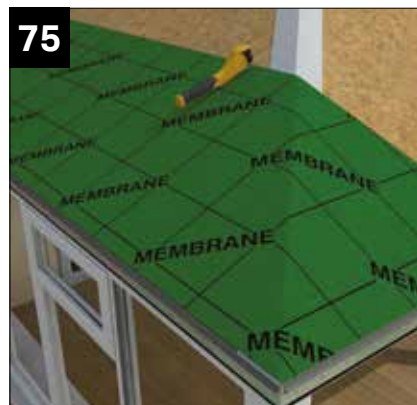
Minimum 200mm overlap over hips. Fix using staple hammer with maximum 12mm stainless steel staples. Take care not to cut through lower layers whilst trimming.
