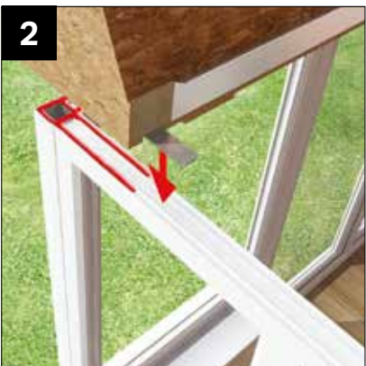
Apply low modulus silicone to the head of frames local to beam area before lifting the box beam into position. Temporarily fix the box beam in position.
