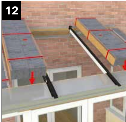
Having installed each gable end panel ensuring each side of the panel is flush with the end of the box beam, continue to install standard (yellow labelled) panels before fitting expandable (red labelled) panels.
